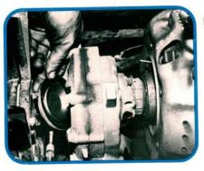
Remove the clamp holding this front cover on the transfer gear housing, then the cover and its seal. Note the location of the breather hole in the cover. A clogged breather will build pressure in the transaxle and cause leaks. Remove the plastic impeller (oil slinger) on the end of the clutch shaft.
