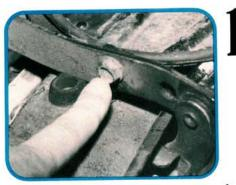
Since all of the work we're going to be doing is right in the front of the engine compartment, the time it takes to remove the hood is time well spent. Remove the washer hose, then remove one bolt from each hinge. Get help removing the hood. It won't realign too well if you drop it. Disconnect the battery for safety's sake.
