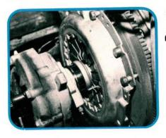
Transfer the retaining ring tool to the new pressure plate. The revised finger design on the new pressure plate makes it easier to remove and install the retaining ring tool. Lower the plate, disc, bearing, and slave cylinder into position. Loosely attach the pressure plate to the flywheel with two top bolts.
